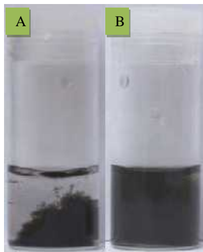
Figure 4. The images of MWNT-COOH and MWNT- Histidine Derivative in deionized water (1mg/6ml) after standing for 1 month.
